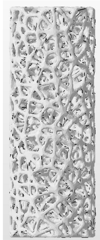
Voronoi Lattice Based Structure
